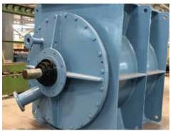
The body & rotor wears out due to heavy handling of material & it's abrasiveness. The gap between rotor blades & body increases making it difficult to control feed rate and smooth operation of rotor.
